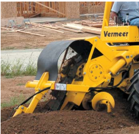
Trencher. The hydrostatic driven center mount trencher has a maximum digging depth of 72" (183 cm) and width of 18" (46 cm).
