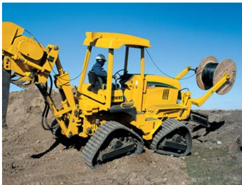
Quad tracks. Features that are available on rubber tire units, such as tilt, four-wheel steer, and crab steering, are functional with the quad tracks. The quad track design has relatively no break-over point and maximizes tractive effort and stability by maintaining constant four-point ground contact.
