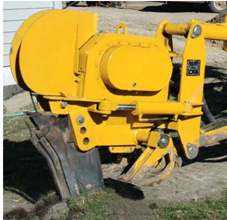
Plow attachment. Attachment installs product up to 36" (91 cm) in depth with a maximum shaker force of 35,906 lb (16,287 kg) and a 30-degree swing angle.
