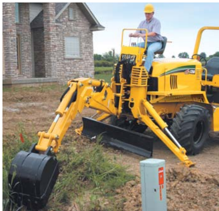
Backhoe. Features a maximum digging depth of 107" (272 cm) with a swing arc of 180 degrees.
