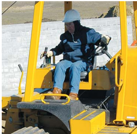
Swiveling operator's console. Hydraulic controls rotate with the operator seat to enhance ease of operation and visibility of the rear attachment.
