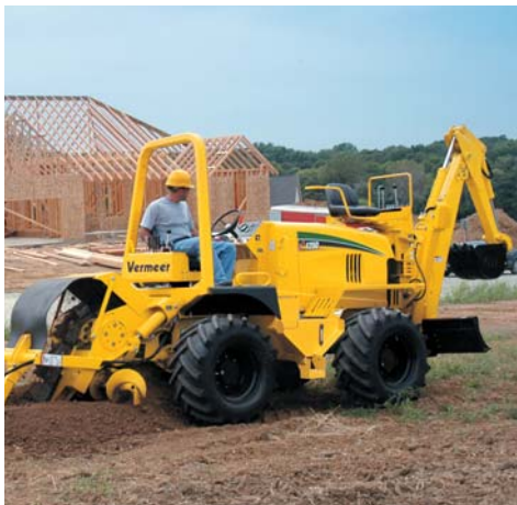
Interchangeable. The RTX1250 design allows the operator to switch between rubber tires or rubber quad tracks to match the unit to the job application and ground conditions.
