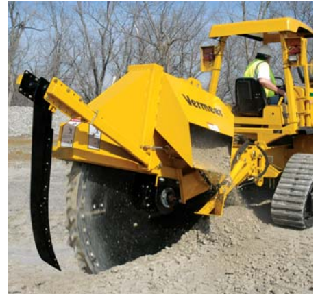
Rockwheel. The hydrostatic driven rockwheel attachment has a maximum cutting depth of 40" (102 cm) and features dual discharge chutes.
