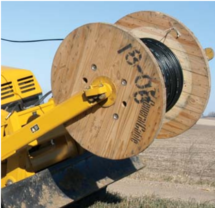
Reel carrier. A 2.5" (6.4 cm) diameter reel shaft supports up to a 3000 lb (1361 kg) reel and offers ease loading capabilities.
