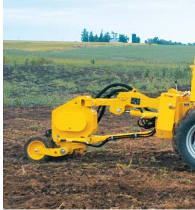
Plow. Attachment installs product up to 36" (91.4 cm) in depth with a maximum shaker force of 24,000 lb (10,886 kg) and a 30-degree swing angle.
