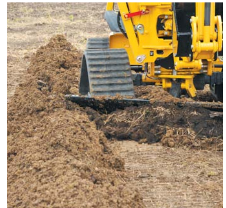
Backfill blade. The blade has a width of 79" (201 cm) with quad tracks, 72" (182.9 cm) with tires, a 30-degree swing angle and a tilt angle of 12 degrees.
