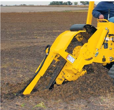
Trencher. The hydrostatic-driven center-mount trencher has a maximum digging depth of 60" (152.4 cm) and width of 12" (30.5 cm).
