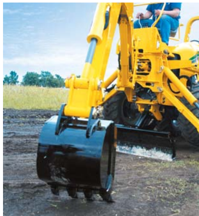
Backhoe. Features a maximum digging depth of 96.8" (245.9 cm) with a swing arc of 170 degrees.
