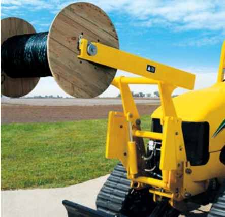
Reel carrier. A 2.25" (5.7 cm) diameter reel shaft supports up to a 1500 lb (680.4 kg) reel.
