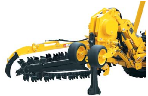
Combo trencher/plow. Multi-use rear attachment can plow depths up to 30" (76.2 cm) and trench depths up to 60" (152.4 cm).
