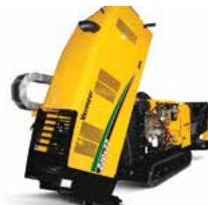
**SERVICEABILITY.** The drill's flip-up metal hood offers ease of access when performing routine service and maintenance.
